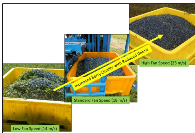
Increase in berry cleanliness with increase in blower fan speed.
