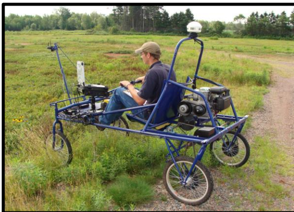
Configuration of automated yield monitoring system mounted on farm motorized vehicle.
