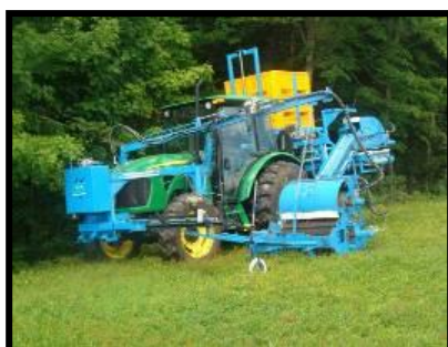
Yield monitoring system, ultrasonic sensor and RTK-GPS incorporated into harvester
